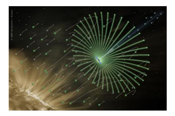
The electric sail (ESAIL), invented by Dr. Pekka Janhunen at the Finnish Kumpula Space Centre in 2006, produces propulsion power for a spacecraft by utilizing the solar wind. The sail features electrically charged long and thin metal tethers that interact with the solar wind. Using ultrasonic welding, the Electronics Research Laboratory at the University of Helsinki successfully produced a 1 km long ESAIL tether.
