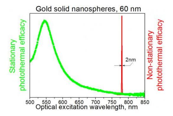
The strong response of plasmonic gold nanoparticles to pulsed ("nonstationary") lasers rather than continuous ("stationary") excitation by lasers appears to be due to the influence of nanobubbles on the particles, according to researchers at Rice University. Credit: Lapotko Group/Rice University
