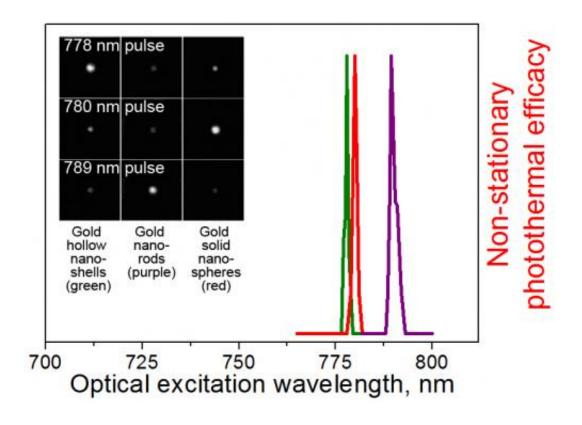
Different types of nanoparticles – in this case, shells, rods and solid spheres – mixed together can be activated individually with pulsed laser light at different wavelengths, according to researchers at Rice University. The tuned particles' plasmonic response, enhanced by nanobubbles that form at the surface, can be narrowed to a few nanometers under a spectroscope and are easily
