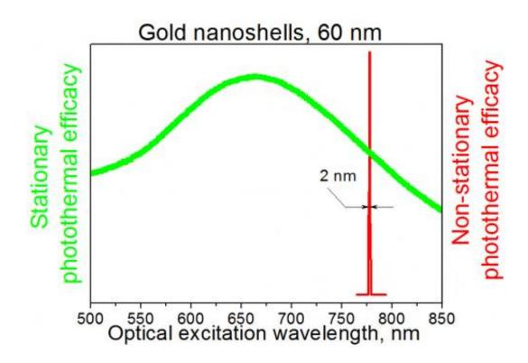
Rice University researchers found that pulsed (or "nonstationary") lasers could narrow the response spectra of 60-nanometer-wide gold nanoshells to a very narrow spectral band (red peak), as opposed to continuous ("stationary") excitation by laser (green peak). The discovery opens new possibilities for the use of metallic nanoparticles in medical and electronic applications. Credit: Lapotko Group/Rice University
