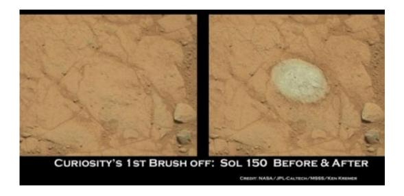
Before and after comparison of images of 1st ever rock brush off by Curiosity's Dust Removal Tool (DRT) on Sol 150 (Jan 6, 2013), nearby to Snake River. Images taken by the high resolution Mastcam 100 camera, contrast enhanced. The brushed patch of rock target called "Ekwir\_1" 'is about 1.85 inches by 2.44 inches (47 millimeters by 62 millimeters). Credit: NASA/JPL-Caltech/MSSS/Ken Kremer
