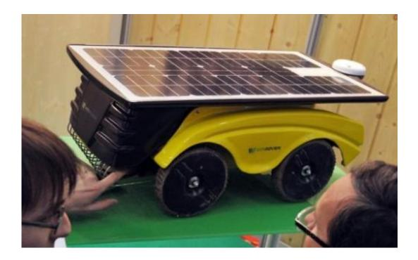
A new solar-powered vineyard robot called Vitirover is displayed on November 27, 2012 at the Vinitech professional wine fair in Bordeaux, southwestern France. Fitted with a GPS receiver and solar panels, the all-land mower Vitirover aims at lightening wine's impact on the soil, by mowing the wild plants between vine rows without the need for heavy, polluting tractors or herbicides.
