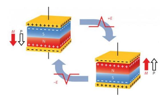
Switching magnetism. In the material studied the magnetic moment (M) and the electrical polarization (P) are coupled, so that negative electrical charges (-) accumulate near the magnetic southpole (S), and positive ones near the northpole (N). By applying an electric voltage (E), the direction of M and P can be reversed. Credit: 2012 Yusuke Tokunaga, RIKEN Advanced Science Institute
