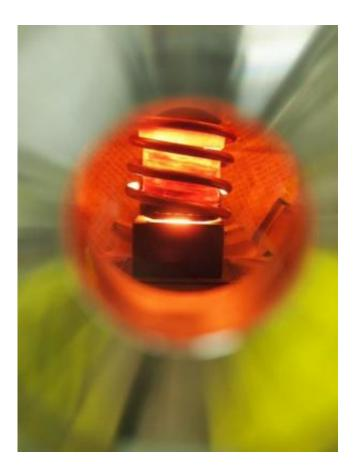
Looking into the high temperature furnace at the induction coil that heats the samples and fixed points.
