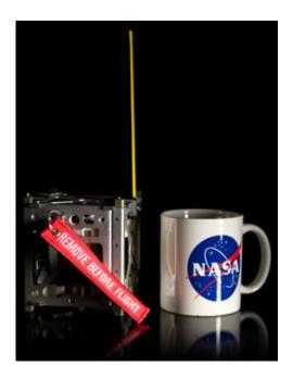
Size of a NASA coffee cup! A trio of CubeSats makes up the innovative PhoneSat Project to be launched next year. Credit: NASA Ames Research Center
