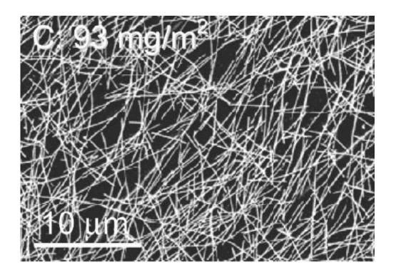
The nanowires have diameters around 0.1 micrometers and lenghts between 5 and 10 micrometers. Credit: Bild: *ACS Nano* 3: 1767-1774
