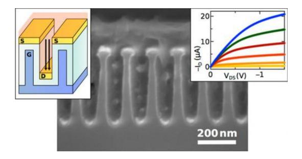
Schematic drawing and scanning electron microscope cross-sectional image of a vertical channel polymer semiconductor field-effect transistor. The device current output (ID) versus voltage (VDS) graph illustrates near-ideal transistor performance attributes at only one-volt operating voltage.
