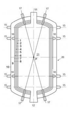
Schematic section of the vessel and the containment wall of the fusion reactor that show the essential components.
