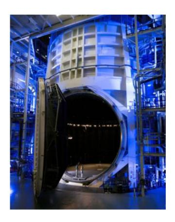
Johnson Space Center's Chamber A is a 16.8 m (55 ft) diameter x 27.4 m (90 ft) high, thermal-vacuum test facility and is famous for testing the Apollo spacecraft, with and without the mission crew. Credit: NASA Johnson
