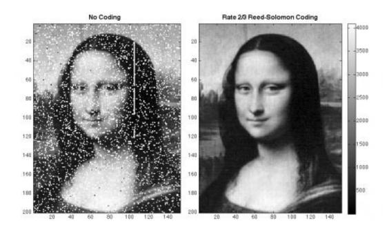
To clean up transmission errors introduced by Earth's atmosphere (left), Goddard scientists applied Reed-Solomon error correction (right), which is commonly used in CDs and DVDs. Typical errors include missing pixels (white) and false signals (black). The white stripe indicates a brief period when transmission was paused. Credit: Image courtesy: Xiaoli Sun, NASA Goddard
