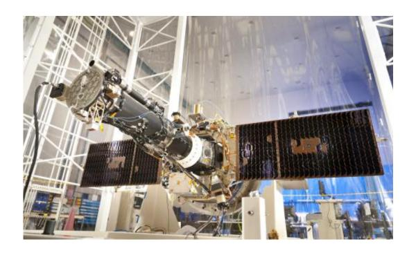
The fully integrated spacecraft and science instrument for NASA's Interface Region Imaging Spectrograph (IRIS) mission is seen in a clean room at the Lockheed Martin Space Systems Sunnyvale, Calif. facility. The solar arrays are deployed in the configuration they will assume when in orbit. Credit: Lockheed Martin
