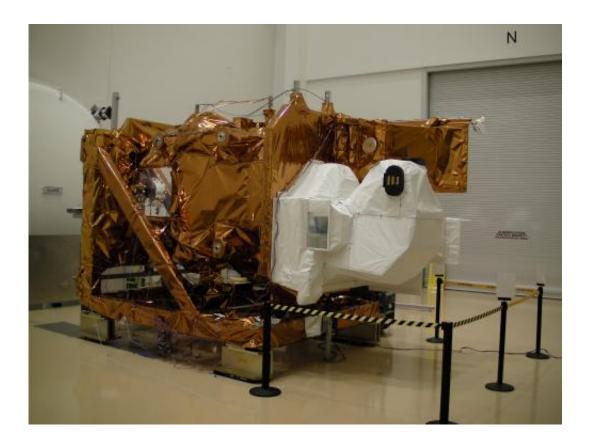
LDCM installed on horizontal support frame after completing thermal vacuum testing at Orbital Sciences Corporation's facility in Gilbert, Ariz. Credit: Orbital
