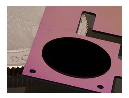
The circular patch of carbon nanotubes on a pink silicon backing is one component of NIST's new cryogenic radiometer, shown with a quarter for scale. Gold coating and metal wiring has yet to be added to the chip. The radiometer will simplify and lower the cost of disseminating measurements of laser power. Credit: Tomlin/NIST
