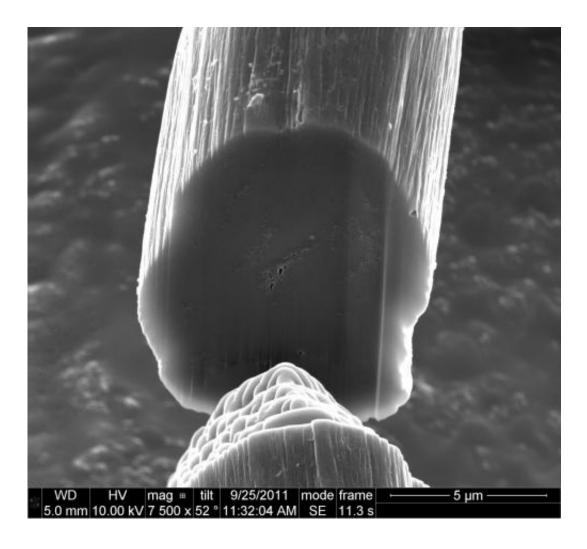
Nanotubes are tightly packed in the new carbon nanotube fibers produced by Rice University and Teijin Aramid. This cross section of a test fiber, which was taken with a scanning electron microscope, shows only a few open gaps inside the fiber. CREDIT: D. Tsentalovich/Rice University
