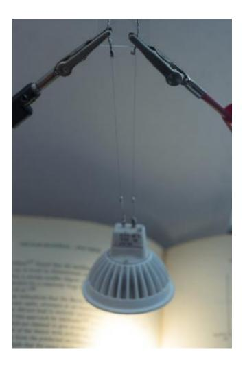
This light bulb is powered and held in place by two thin strands of carbon nanotube fibers that look and feel like textile thread. The nanotube fibers conduct heat and electricity as well as metal wires but are stronger and more flexible. CREDIT: Jeff Fitlow/Rice University
