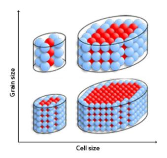
Phase change in NGST is faster when the grains are smaller and arranged into tinier cells, owing to an increase in the ratio of surface (blue) to internal (red) grains and the interface between grains. © 2012 Nature Publishing Group
