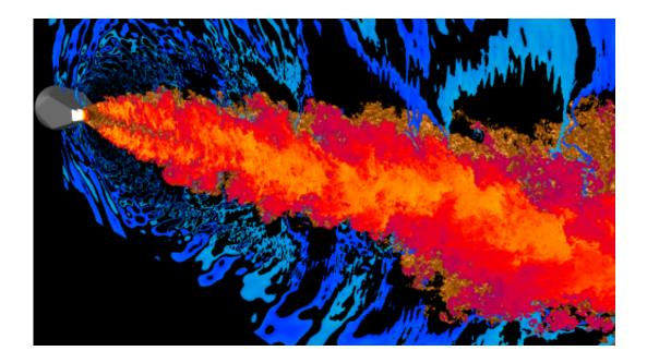
This is an image from the jet noise simulation. A new design for an engine nozzle is shown in gray at left. Exhaust temperatures are in red/orange. The sound field is blue/cyan. Chevrons along the nozzle rim enhance turbulent mixing to reduce noise. Credit: Courtesy of the Center for Turbulence Research, Stanford University
