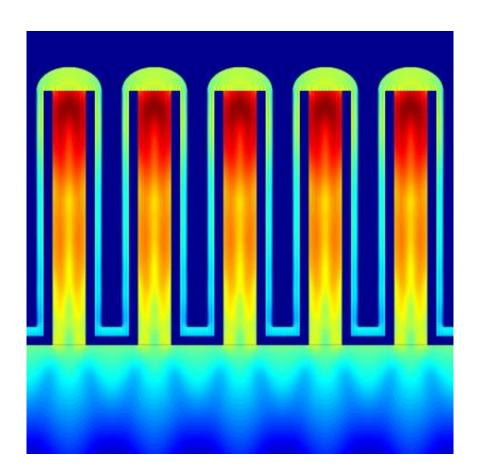
This shows a computer simulation of the absorption in five nanowires. The
