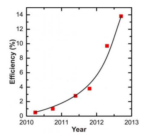
This shows the photovoltaic efficiency of millimeter square InP single band gap nanowire solar cells as a function of time measured within the FP7 financed AMON-RA project. About four million InP NWs contribute to the signal. The line is a guideline for the eye. This figure gives an overview of the development of NWPV within AMON-RA. A comparison with the record efficiency
