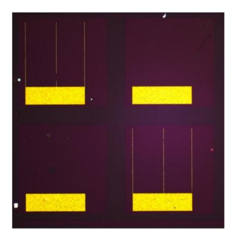
This shows an optical microscope image of four nanowire solar cells. Each cell is a slightly lighter shade of purple in color, while the darker areas in between are inactive. The yellow areas are gold metal pads, which are used for connecting the solar cells to an external load. Each cell contains about 4.5 million nanowires. Credit: Wallentin et al.
