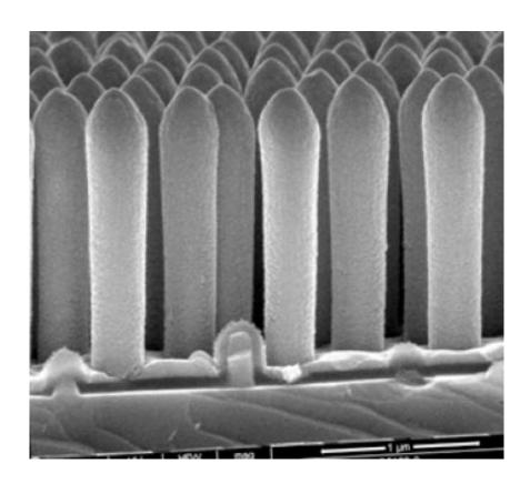
This scanning electron microscopy (SEM) image shows a side-view of nanowires which have been coated with a transparent and conductive oxide. The sunlight comes in from top, which is why the top contact must be transparent for light. The substrate is used for the bottom contact. Credit: Wallentin et al.
