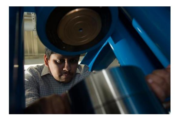
Rice University geologist Rajdeep Dasgupta uses powerful hydraulic presses to crush rock samples in pressures that simulate those found deep inside the Earth. New research by Dasgupta and his colleagues revealed that magma can form much deeper in the planet's mantle than previously thought. Credit: Jeff Fitlow/Rice University
