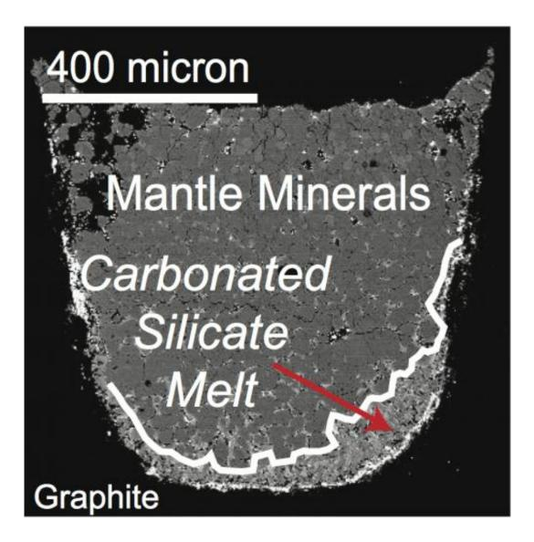
A microscopic sample of rock squeezed in a lab at Rice University to pressures it would experience hundreds of kilometers inside the Earth's mantle show evidence of magma (silicate melt) formation. New research led by Rice shows magma can form as deep as 250 kilometers inside the mantle. Credit: Dasgupta Group/Rice University
