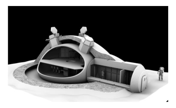
For ESA's 3D-printed lunar base concept, Foster+Partners devised a weightbearing 'catenary' dome design with a cellular structured wall to shield against micrometeoroids and space radiation, incorporating a pressurised inflatable to shelter astronauts. Credit: ESA
