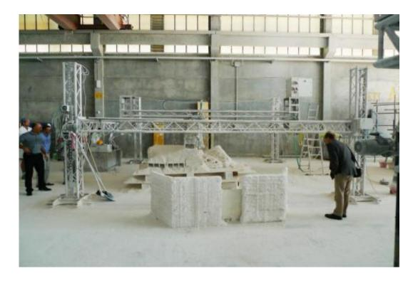
The UK's Monolite supplied the D-Shape printer for ESA's 3D-printed lunar base study, with a mobile printing array of nozzles on a 6 m frame to spray a binding solution onto a sand-like building material. 3D 'printouts' are built up layer by layer – the company more typically uses its printer to create sculptures and is working on artificial coral reefs to help preserve beaches from energetic sea waves. First the simulated lunar material with magnesium oxide – turning it
