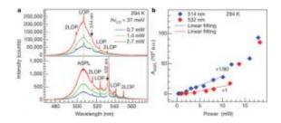
Multiple-LOP-assisted up-conversion spectra of CdS nanobelts. Credit: *Nature* 493, 504–508, doi:10.1038/nature11721
