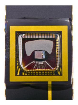
Strong performance: During tests, the organic sensors proved to be up to three times more sensitive to light than conventional CMOS sensors. Credit: Photo: A. Heddergott / TUM
