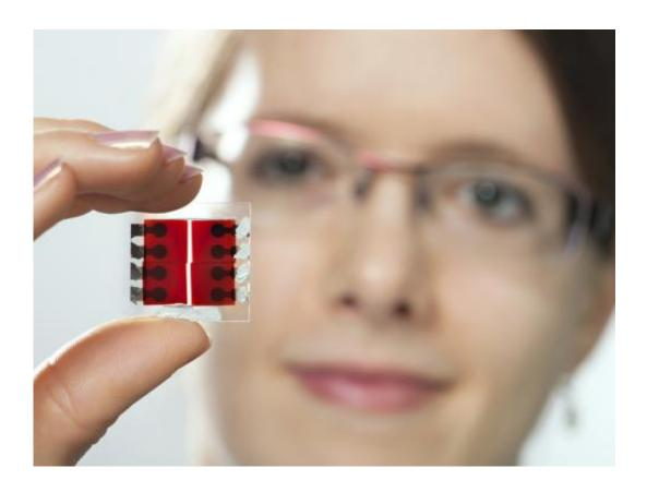
Ultra-thin: Organic sensors can be applied to CMOS chips over large and small surfaces, as well as to glass or flexible plastic films. Credit: Photo: U. Benz / TUM
