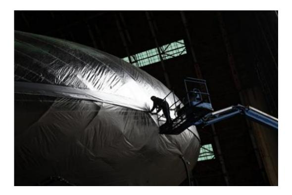
Leonel Cruz pulls down the flab on the Aeroscraft airship, a high-tech prototype airship, in a World War II-era hangar in Tustin, Calif., Thursday, Jan. 24, 2013. Work is almost done on a 230-foot rigid airship inside a blimp hangar at a former military base in Orange Co. The huge cargo-carrying airship is has shiny aluminum skin and a rigid, 230-foot aluminum and carbon fiber skeleton. (AP Photo/Jae C. Hong)
