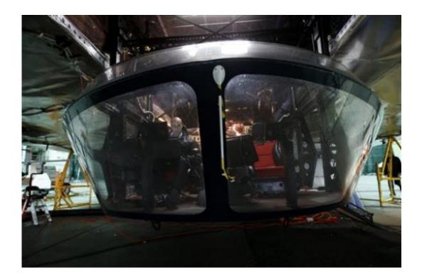
Aerospace engineer Munir Jojo works in the cockpit of the Aeroscraft airship, a high-tech prototype airship, in a World War II-era hangar in Tustin, Calif., Thursday, Jan. 24, 2013. Work is almost done on a 230-foot rigid airship inside a blimp hangar at a former military base in Orange Co. The huge cargo-carrying airship is has shiny aluminum skin and a rigid, 230-foot aluminum and carbon fiber skeleton. (AP Photo/Jae C. Hong)
