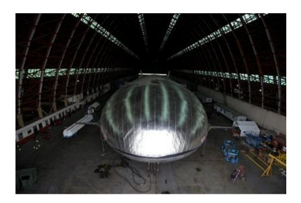
The Aeroscraft airship, a high-tech prototype airship, is seen in a World War II-era hangar in Tustin, Calif., Thursday, Jan. 24, 2013. Work is almost done on a 230-foot rigid airship inside a blimp hangar at a former military base in Orange Co. The huge cargo-carrying airship is has shiny aluminum skin and a rigid, 230-foot aluminum and carbon fiber skeleton. (AP Photo/Jae C. Hong)
