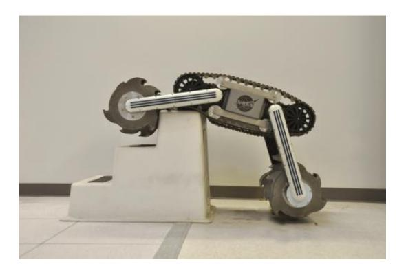
The RASSOR can climb over a large obstacle, such as a boulder on the moon. Engineers on Earth used a stepping stool to challenge the robot. Credit: NASA
