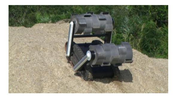
The RASSOR robot climbs a hill during recent testing at NASA's Kennedy Space Center in Florida. Credit: NASA
