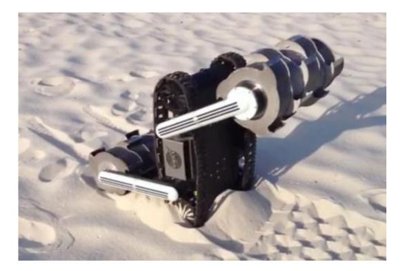
With a pair of drums positioned on arms, the RASSOR can take on a number of different shapes to accomplish its work. Credit: NASA
