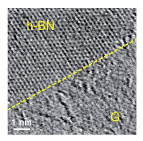
A scanning transmission electron microscope image shows a razor-sharp transition between the hexagonal boron nitride domain at top left and graphene at bottom right in the 2-D hybrid material created at Rice University. Credit: Oak Ridge National Laboratories/Rice University
