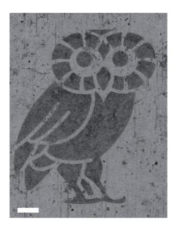
An atom-thick Rice Owl (scale bar equals 100 micrometers) was created to show the ability to make fine patterns in hybrid graphene/hexagonal boron nitride (hBN). In this image, the owl is hBN and the lighter material around it is graphene. The ability to pattern a conductor (graphene) and insulator (hBN) into a single layer may advance the ability to shrink electronic devices. Credit: Zheng Liu/Rice University
