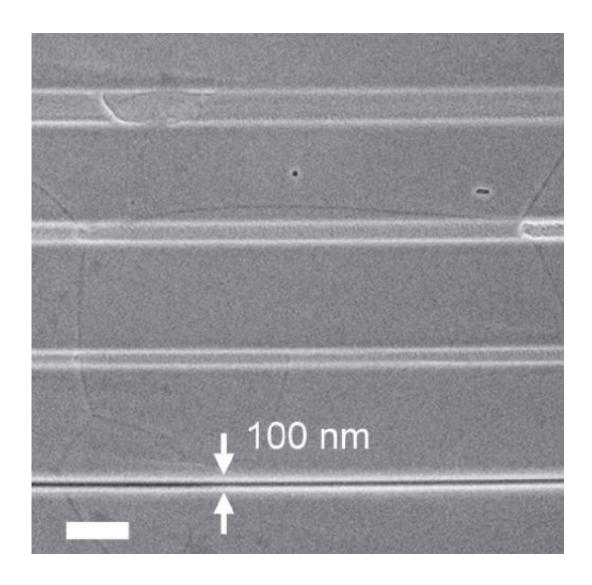
A photolithography process was used at Rice University to develop a patterned, one-atom-thick hybrid of graphene and hexagonal boron nitride (hBN). Graphene is a conductor and hBN is an insulator, so the 2-D material has unique
