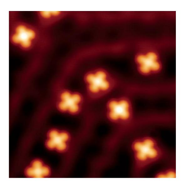
A scanning-electron micrograph of iron-phthalocyanine molecules (seen as bright crosses) adsorbed on a gold surface. The image size is 15 x 15
