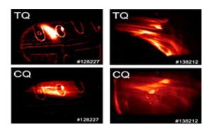
Thermal quench (TQ) and current quench (CQ) studies are part of the research underway on disruption mitigation and runaway electron suppression. Credit: General Atomics
