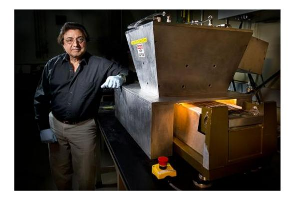
NREL scientist Bhushan Sopori stands beside the Silicon Photovoltaic Wafer Screening System, which puts thermal pressure on wafers to determine if they will survive the rigors of turning them into solar cells. Credit: Dennis Schroeder
