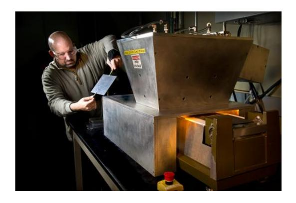
NREL postdoctoral scientist Rene Rivero readies a wafer for the Silicon Photovoltaic Wafer Screening System. Credit: Dennis Schroeder
