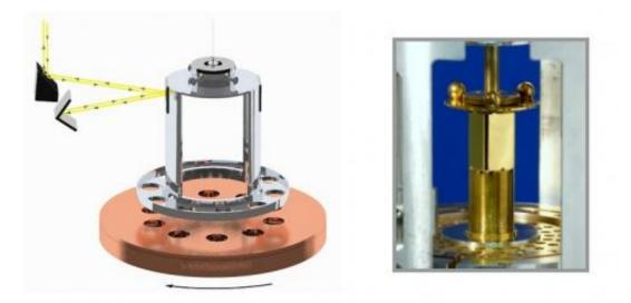
The Eöt-Wash experiment may test for Upadhye's predicted torque signal due to the symmetron field. A fifth force could be measured in the submillimeter distance between the two disks. (Left) An illustration of an older model and (right) a photo of a newer instrument. Credit: The Eöt-Wash Group at the
