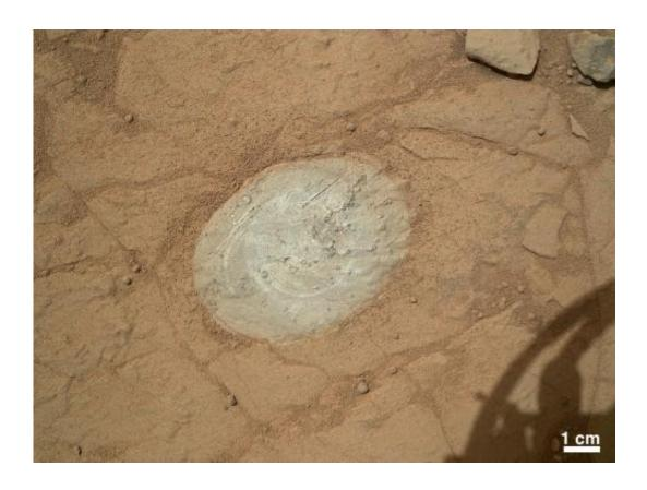
This image from the Mars Hand Lens Imager (MAHLI) on NASA's Mars rover Curiosity shows the patch of rock cleaned by the first use of the rover's Dust Removal Tool (DRT). Credit: NASA/JPL-Caltech/MSSS
