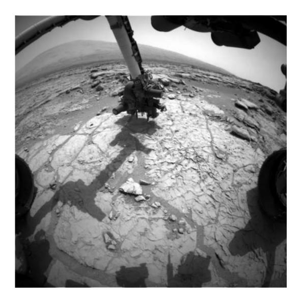
The percussion drill in the turret of tools at the end of the robotic arm of NASA's Mars rover Curiosity has been positioned in contact with the rock surface in this image from the rover's front Hazard-Avoidance Camera (Hazcam). Credit: NASA/JPL-Caltech
