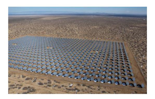
This aerial view of the solar photovoltaic array at White Sands Missile Range, N.M., was taken, Jan. 8, 2013. The panels cover 42 acres and provide more than four megawatts of electricity to the base. Credit: Solaria
