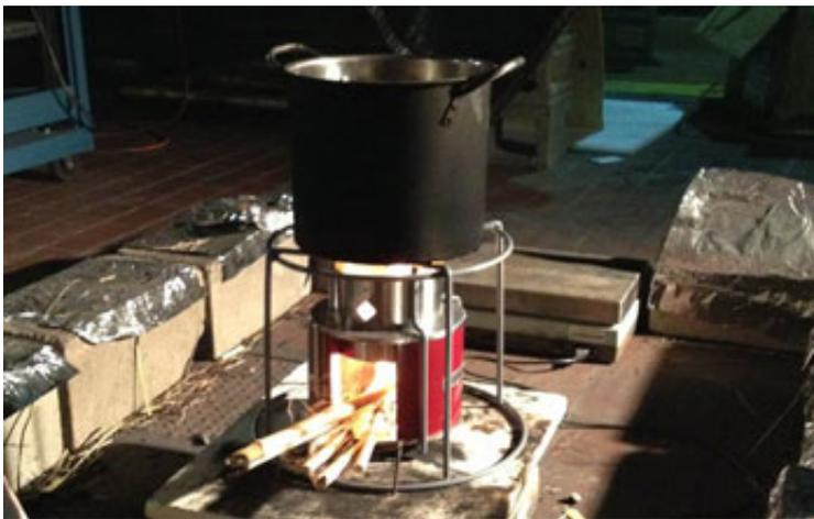
A lab tests emissions from the new EZY stove using millet stalks as fuel. Credit: Gavin McMeeking
