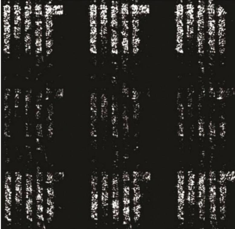
Because of the interference of the phase-shifted light beams emitted by the antennas, images of the MIT logo appear to hover above the surface of the chip.
