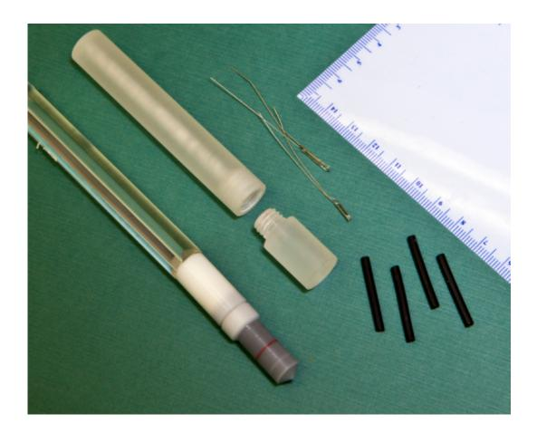
From bottom left: an ionization chamber in its casing, a polystyrene enclosure for thermistors, and two thermistors. The black items at right are thermistor covers.
