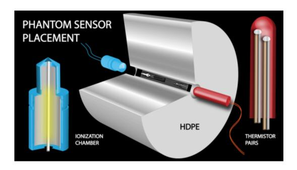
Schematic diagram of sensor placement in phantom. In the center channel is an actual x-ray image of an ionization chamber (left) and thermistors (right) within an HDPE phantom.
