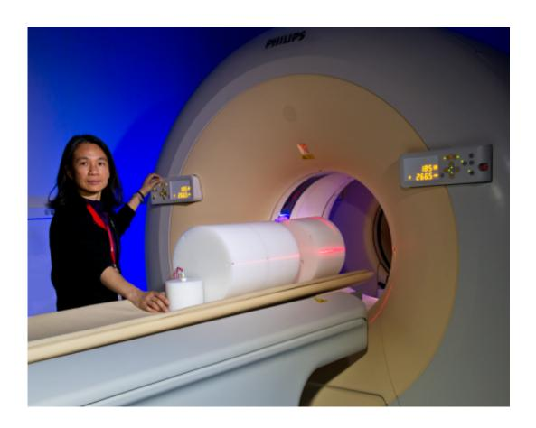
Heather Chen-Mayer in front of PML's PET/CT scanner with HDPE phantoms. The large sections are for whole-torso measurements, the small one for an adult head.
