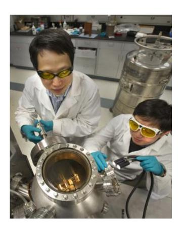
Brookhaven physicists Weidong Si (left) and Qiang Li look into the vacuum chamber where the new high-field iron-based superconductors are made through a process called pulsed-laser deposition.
