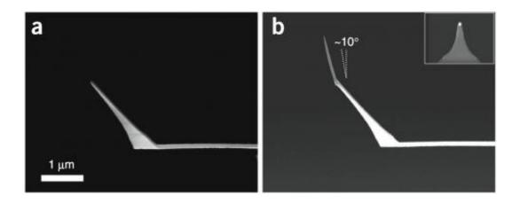
Scanning electron microscope images show two different designs of cantilever tip used by Ando and co-workers for high-speed atomic force microscopy.
