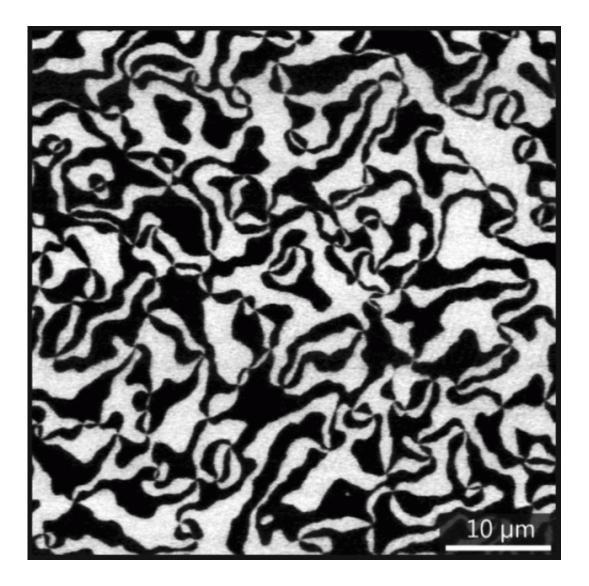
Regions with different orientation of the electric charges in yttrium manganite (white and black areas correspond to a positiver and negative charge distribution, respectively). The star-shaped intersections where bright and dark regions meet are the defects corresponding to the cosmic strings.
