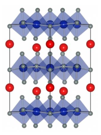
Structure of the yttrium manganite crystal. The figure shows the atomic unit cell from which the investigated crystals are composed. Manganese atoms (blue) are placed within a cage of oxygen atoms (gray). In between these the yttrium atoms (red) are arranged. The slight tilt of the oxygen cages to the left or right is the basis of the phase transition described in the text.
