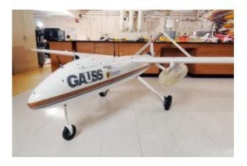
The GTRI Airborne Unmanned Sensor System (GAUSS) is used to evaluate sensing devices in airborne testing. Credit: Gary Meek
