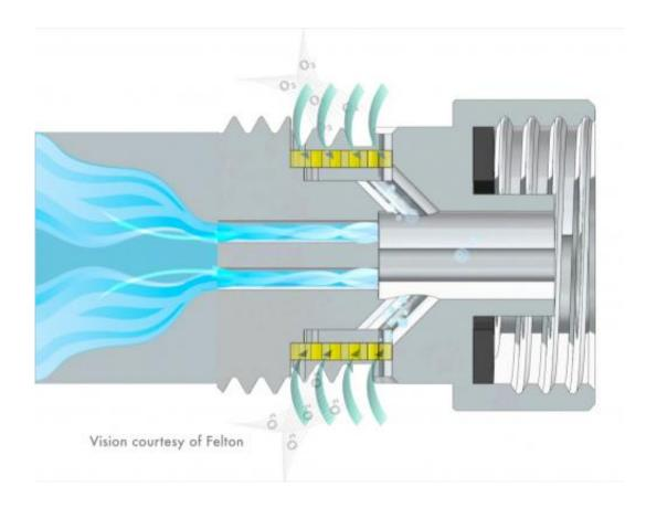
The nozzle draws air into the water flow, making the water droplets hollow. Credit: Felton
