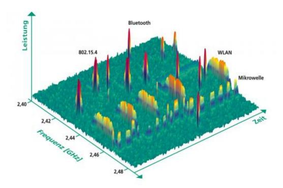
Awair? displays when signals are being transmitted and on which frequencies. Credit: © Fraunhofer ESK
