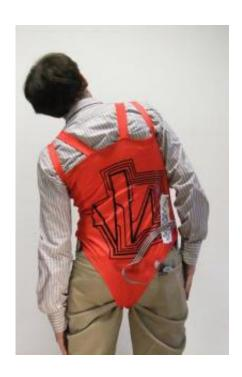
Neurorehabilitation researchers from Italy have developed a low cost, wearable system, consisting of strain sensors made of conductive elastomers printed onto fabric. Credit: Paolo Tormene
