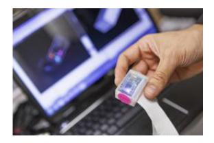
A wearable wireless sensor can detect precursors of falls. The system would be used for fall prevention in the elderly.
