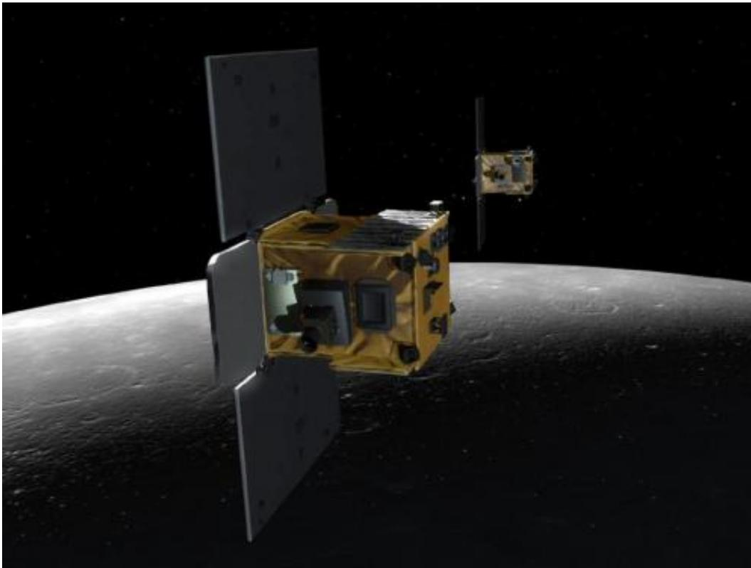
An artist's depiction of the twin spacecraft (Ebb and Flow) that comprise NASA's Gravity Recovery And Interior Laboratory (GRAIL) mission. Credit: NASA/JPL-Caltech/MIT
