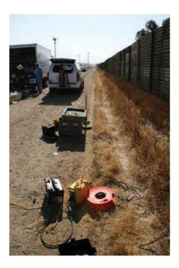
Researchers deploy instruments for a seismic data acquisition survey parallel to a border fence in California. The photo shows some acquisition equipment, including an SUV-mounted accelerated weight drop to generate seismic waves. Credit: courtesy of Sandia National Laboratories
