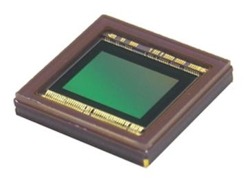
Toshiba Corporation today announced that it will launch a new 20-megapixel (MP) CMOS image sensor, the TCM5115CL, as the latest addition to its sensor line-up for digital still cameras. TCM5115CL offers the industry's highest resolution in the 1/2.3 inch optical format, using backside illumination technology (BSI) to improve sensitivity and imaging performance.
