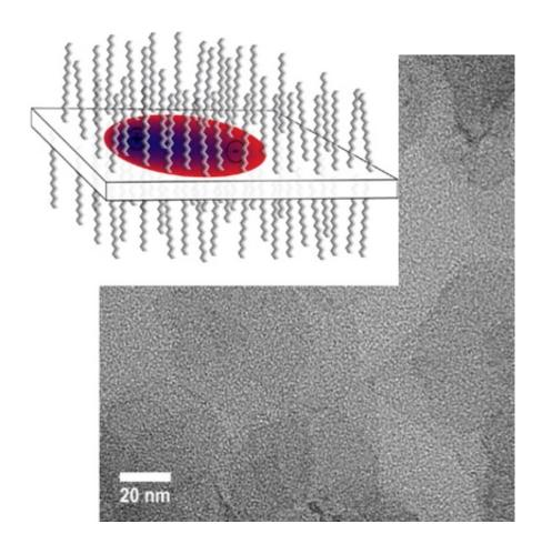
Schematic and transmission electron microscope (TEM) image of CdSe nanoplatelets with a thickness of 5 monolayers.
