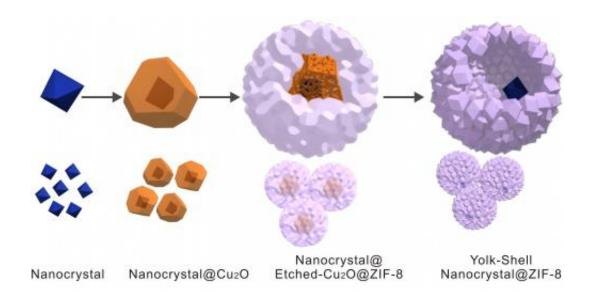
Boston College researches started with a metallic crystal. It was then coated with a "sacrificial layer" of copper oxide. The application of ZIF-8 formed a porous skin that then etched away the copper. Within the resulting cavity, researchers were able to control the chemical reaction thanks to the skin-like shell of ZIF-8. Credit: *Journal of the American Chemical Society*
