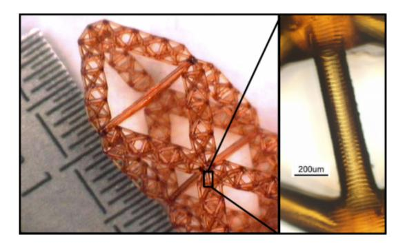
Fractal frame. This construction shows the similarity of different scales ("self-similarity") in a generation-2 hierarchical structure. Due to manufacturing limitations, the scaffolding here is made of solid rather than hollow beams (inset). Credit: D. Rayneau-Kirkhope et al., Phys. Rev. Lett. (2012)
